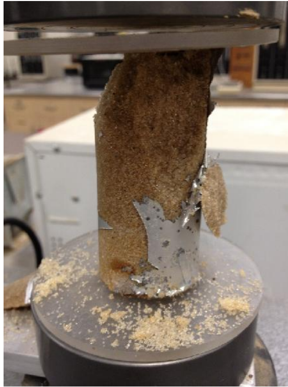
Figure 24. Failed silica sand sample after unconfined compression
