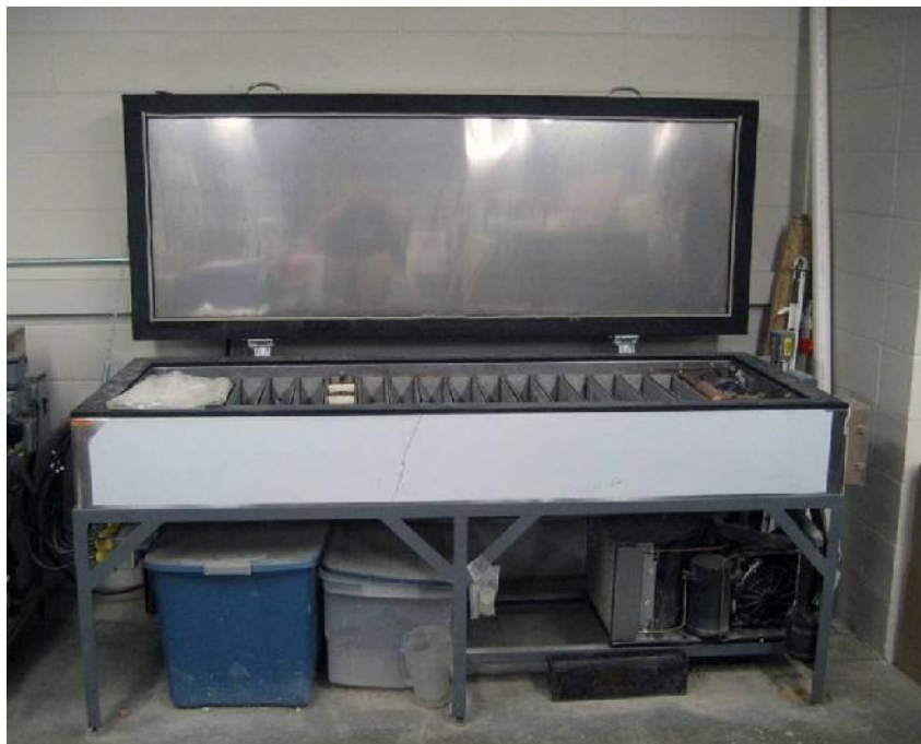
Figure 11. Humboldt H-3185 rapid freeze-thaw cabinet
